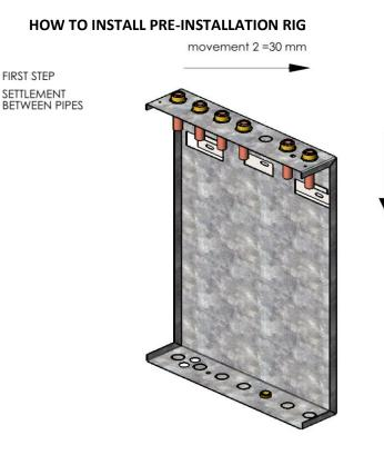
**STEP1:** Securely fix the mounting bracket to the wall in the required position. Hang the ModuSat® XR Pre-Installation Rig on the wall fixing bracket. Then slide down and across to the right, as indicated in diagram.
