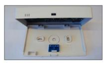
Step 2 Once the tab has been released the cover can be hinged up to access connection
