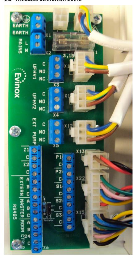
Please Note: When connecting external valves or pumps to the ModuSat control board, it must be ensured that each connection does not exceed 1amp @ 220/240V (AC).
