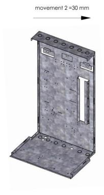
**STEP1:** Securely fix the mounting bracket to the wall in the required position. Hang the ModuSat SPC Pre-Installation Rig on the wall fixing bracket. Then slide down by 15mm and across to the right by 30mm, as indicated in diagram.
