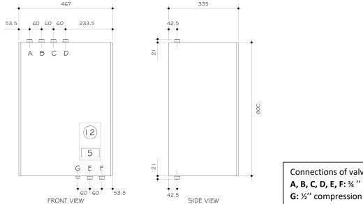
Connections of valve kits: A, B, C, D, E, F: ¾ " BSP int.thread
