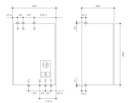
Connections of valve kits: **A, B, C, D, E, F:** ¾ " BSP int.thread **G:** ½" compression
