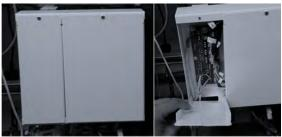
To access the connection board, take off the cover. The retaining screw should be removed and the cover lifted off. The connection board will then be accessible and all required connections can be made simply using the clearly labelled screw down terminal connections. Guides for the various connection applications and requirements are detailed in the wiring principle drawings shown on pages 24-26.
