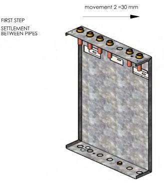
**STEP1:** Securely fix the mounting bracket to the wall in the required position. Hang the ModuSat® XR Pre-Installation Rig on the wall fixing bracket. Then slide down and across to the right, as indicated in diagram.
