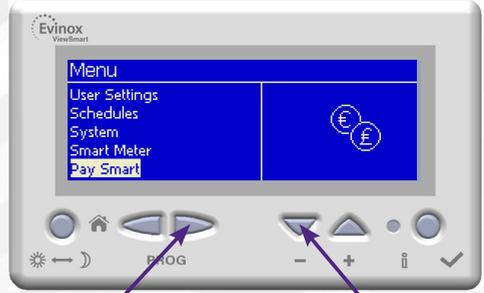
2. Select **"PaySmart"** by scrolling down using the **- button** and pressing the **Right Hand Scroll** button to enter the menu.
