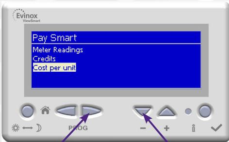
3. Select **Cost per Unit** by scrolling down using the **-** button. Press the **Right Hand Scroll** Button to enter the next screen.
