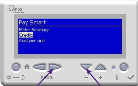
3. Select **Credits** by scrolling down using the **- button**. Press the **Right Hand Scroll** Button to enter the next screen.
