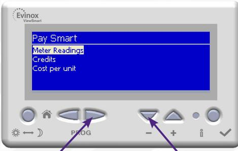
3. Select **Meter Readings** by scrolling down using the **-** button. Press the **Right Hand Scroll** Button to enter the next screen.
