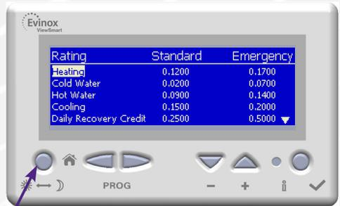
4. The cost per unit is shown for each meter installed in your property. Meters may include-
